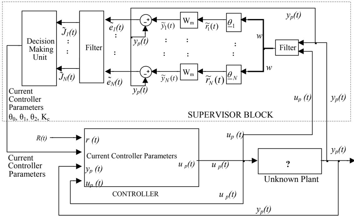
Figure 4: Architecture for control using  $N$  candidate controllers  $\theta_i$ ,  $i = 1, \dots, N$  for MRAC problem
