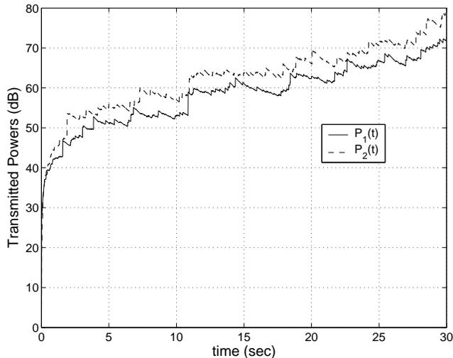
Fig. 6. High fading ( $\sigma = 6$ ); power vectors unbounded
