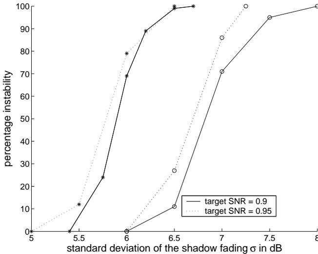
Fig. 3. Percentage instability as a function of standard deviation of fading for  $D_2 = 0.4$  km (\*) and  $D_2 = 0.3$  km (o) and various target SINR
