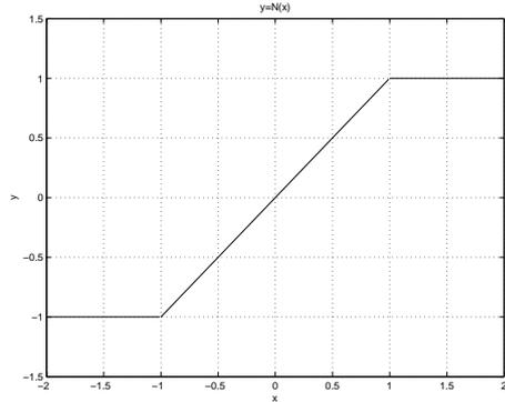
Fig. 2. The saturation nonlinearity  $N(x)$
