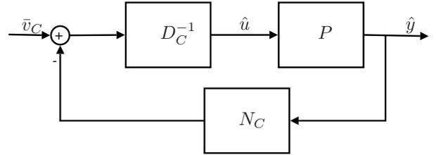
Fig. 3. Virtual closed loop associated to the definition of  $\bar{v}_C(t)$ .
