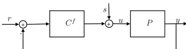
Fig. 5. Figure shows the conventional signals involved in the internal stability proof of a closed loop scheme.
