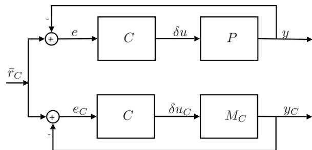
Fig. 7. Double closed loop related to controller  $C$  with the virtual reference signal  $\bar{r}_C$  as the common reference signal.
