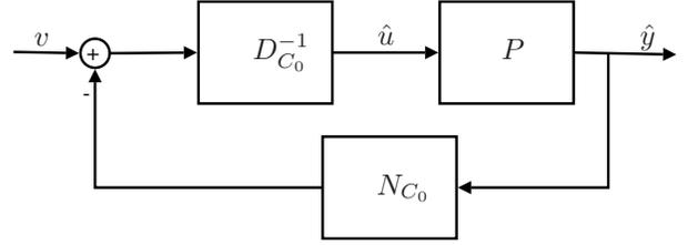
Fig. 2. Operating feedback loop when the controller is written in the MFD form
