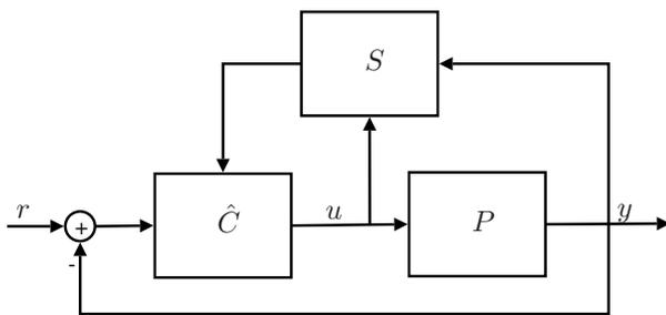
Fig. 1. Basic scheme of an adaptive control system.
