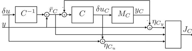
Fig. 8. Figure shows the supervisory logic necessary to produce the cost function  $J_C$  associated to the controller  $C$ .
