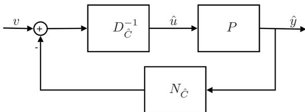
Fig. 4. Adaptive closed loop with the controller written in the MFD form.
