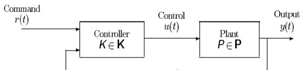
Figure 1: Feedback control system.
