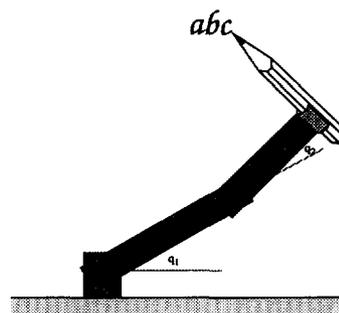
Figure 1: A two-link robot manipulator with joint angles  $q_1(t)$  and  $q_2(t)$ .
