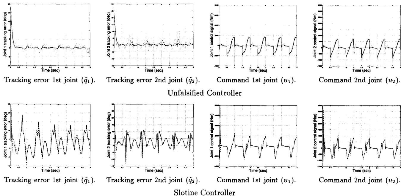
Figure 4: Comparison of tracking errors  $\tilde{q}$  and control signals  $u$  indicates that the unfalsified controller produces a quicker, more precise response, without increased control effort (solid line: ideal actuator, dashed line: 20 hz actuator dynamics, dotted line: 5 hz actuator dynamics).
