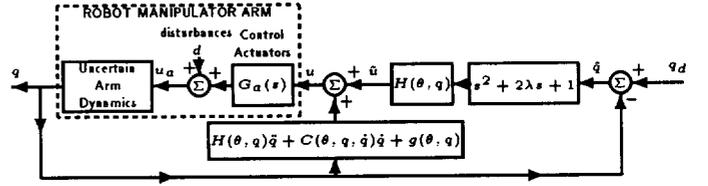
Figure 2: Computed torque manipulator control configuration.
