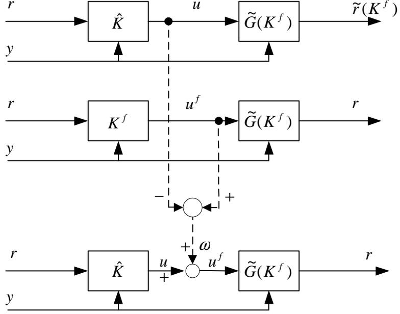
Figure 3.3: Generators of the true and fictitious reference signals.
