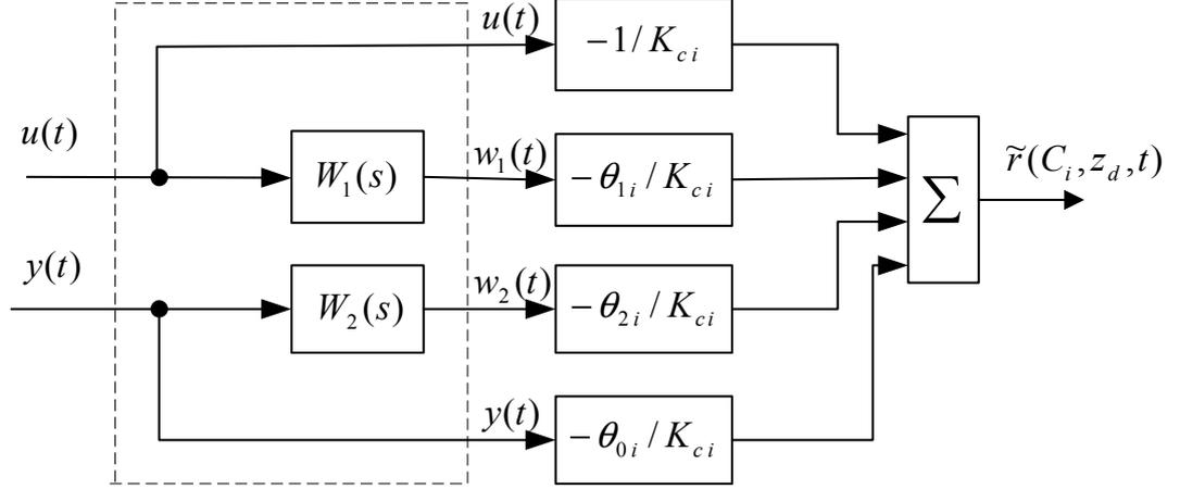
Figure 3.2: Fictitious reference signal of the controller in Fig.3.1
