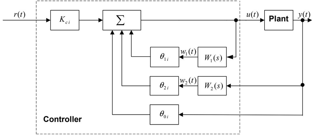
Figure 3.1: A controller with a minimum-phase subsystem from  $r$  to  $u$
