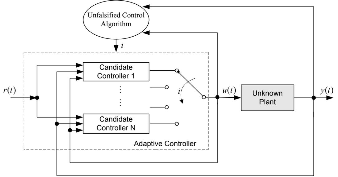
Figure 4.1: Unfalsified adaptive control system using multiple controllers
