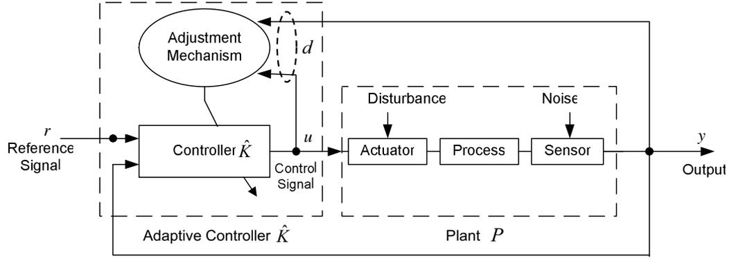
Figure 2.1: Adaptive control system  $\Sigma(P, \hat{K})$
